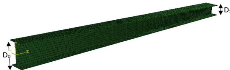
Figure 1: Geometry of linearly tapered w-section member.
