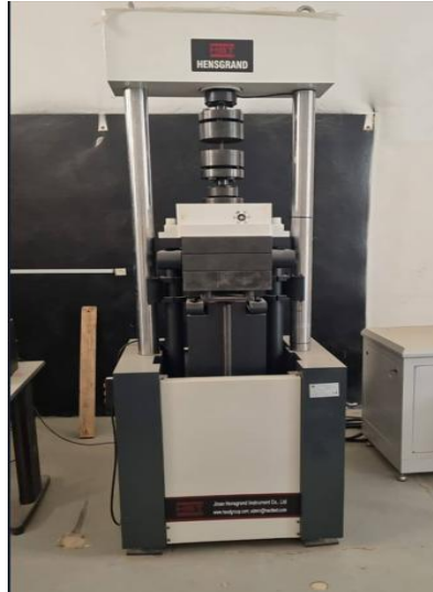
Figure 4: Fatigue test machine used in the study.
