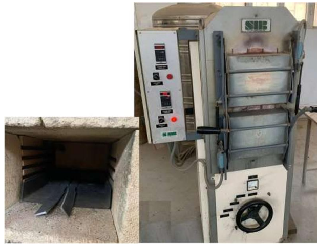
Figure 1: Muffle Furnace used for the heat treatment
